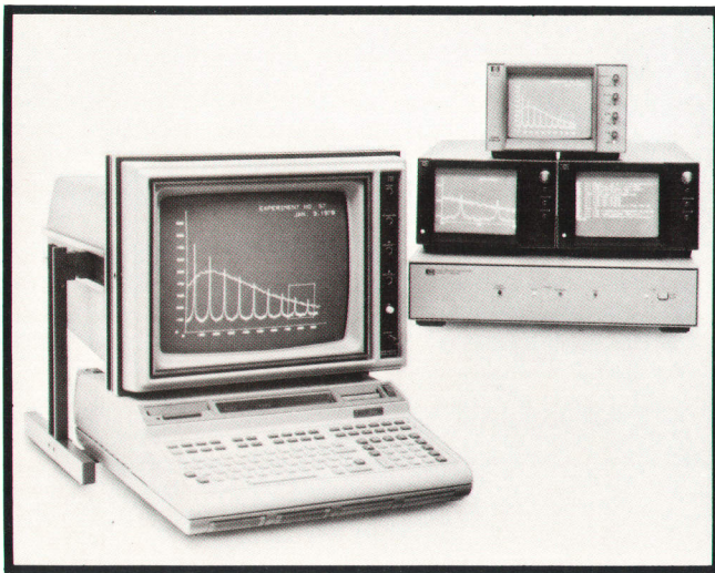
Fig. 8. Graphics work station uses the Model 1350A Graphics Translator with the Model 9825A Desktop Computer. Vectors and characters for all the displays shown here are stored in Model 1350A's files at the same time and directed to individual displays by Model 1350A's blanking signals.
